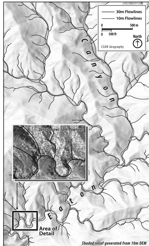
**Figure 2** Flow line models extracted from a 30 metre resolution DEM and a 10 metre resolution DEM. The inset shows both models overlaid onto a 1 metre resolution true colour image
