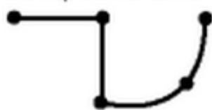
Compound Line String
