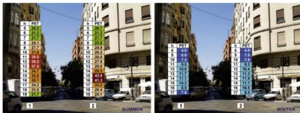
Fig. 10. PET values obtained at different times of the day (h) at the two meteorological stations (shown by points 1 and 2) placed in Cirilo Amorós street.
