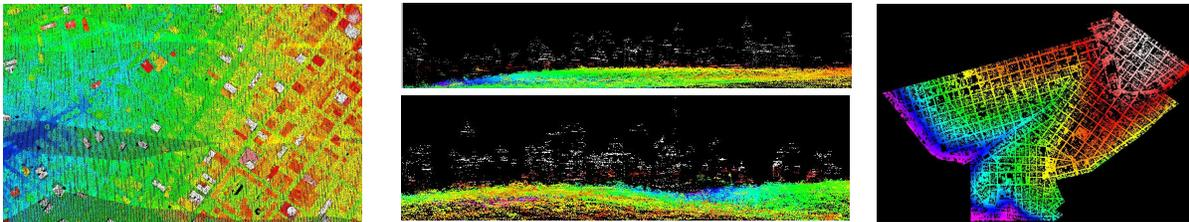
Figure 3.3 – Visualization of the laser data (a) DSM; (b) DSM profiles; (c) DTM.
