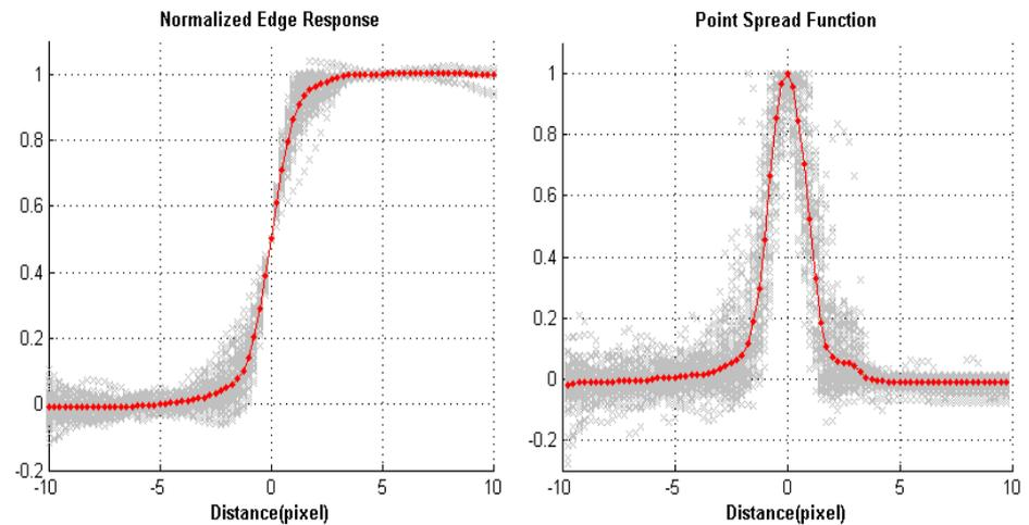
Extracted Edge Profile and Point Spread Function
