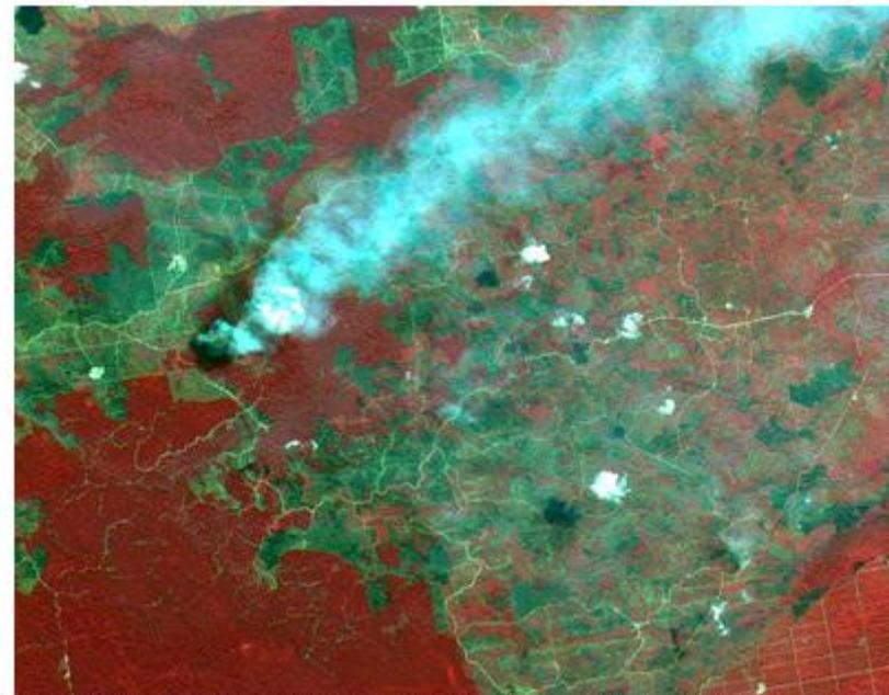
False colour composite of a SPOT 4 multispectral image without displaying the SWIR band:
